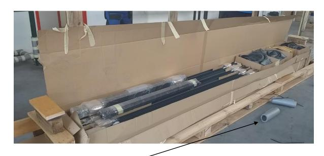
Please keep the <u>grey sponges</u> for later use as a padding underneath the frame / sections / sliding door during the assembly to avoid damages
